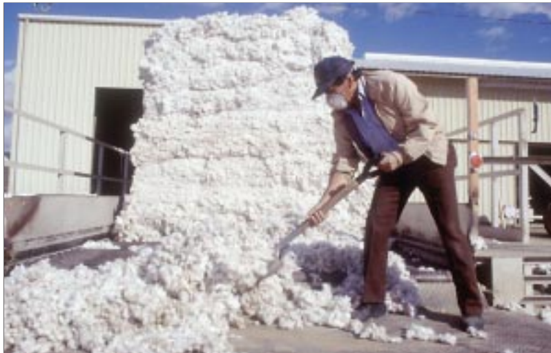
Pima picked too wet can suffer fiber damage in the module. It can sustain further damage when run through the gin's module feeder.
